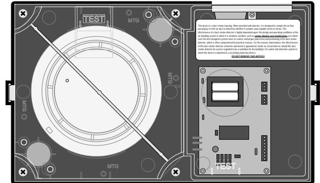
4098-9687 Stand-Alone Duct Detector Housing, Front View
