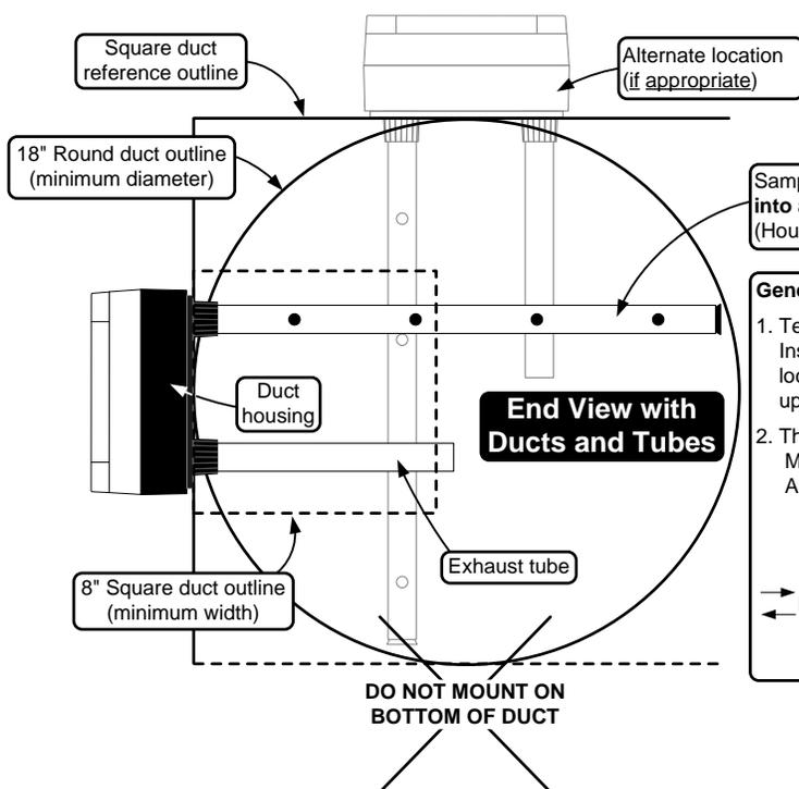
Sampling tube, keyed for proper hole alignment with holes facing into airflow (template is provided for proper tube installation). (Housing is shown as position 2 per note 2 below.)
