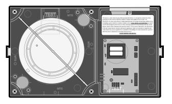
4098-9687 Stand-Alone Duct Detector Housing, Front View
