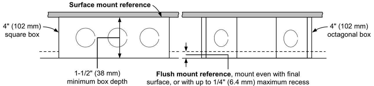
4098-9832 Adapter Plate, required for mounting to surface mounted boxes and to 4" square flush mount boxes
