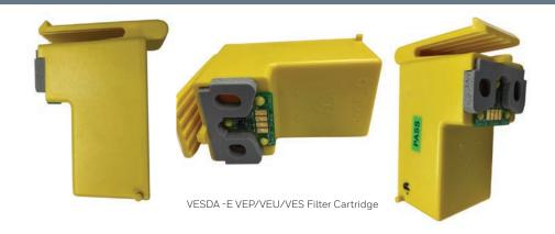
VESDA-E detectors have field replaceable parts, one of which is the filter, VEP/VEU/VES filter part no. VSP-962. The VESDA-E filter cartridge cannot be cleaned and must be replaced with a new one.
