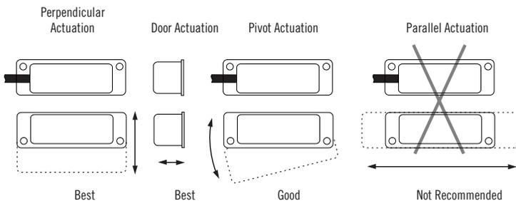
Three configurations are appropriate for interlock applications. The parallel actuation can result in on/off/on signal if the actuator passes by the switch rather than coming to rest in proximity to it. This is NOT a recommended configuration for interlock applications.
