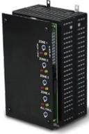
The ANSZM4B2A Zone Splitter Module is used to enable the output of the ANS25, ANS50 or ANS100 to be split into multiple circuits for audio power distribution. The module accepts input from the ANS speaker output and utilizes output relays to distribute the power to separate circuits. The module may be cascaded to increase the number of circuits, and
