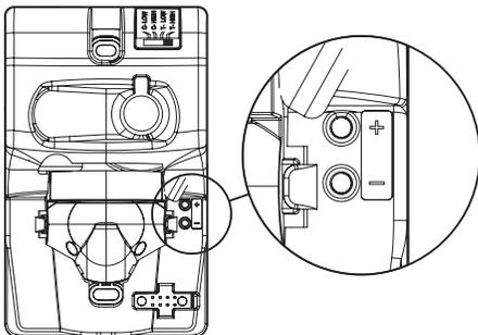
Test points indicated above are used to validate the Notification Appliance Circuit and verify device function.
