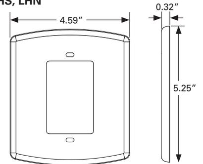
**Note:** For the 4" square backbox, installer must provide a standard metal 4" square one gang device ring to the single gang trim plate.
