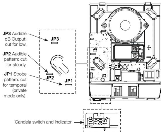
Genesis G4LF Series strobe lights may be set for 15, 30, 75, or 110 candela output. The output setting is changed by simply opening the device and sliding the switch to the desired setting. The appliance does not have to be removed to change the output setting. The setting remains visible through a small window on the side of the device after the cover is closed.
