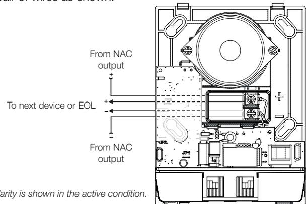
Note: Polarity is shown in the active condition.
