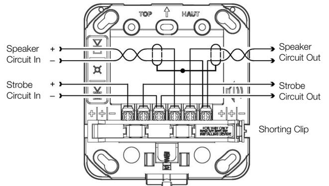
Test points indicated above are used to validate the Notification Appliance Circuit and verify device function.
