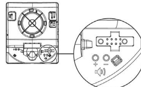
Test points indicated above are used to validate the Notification Appliance Circuit and verify device function.
