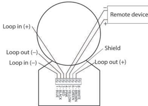
FIGURE 12: Loop wiring
