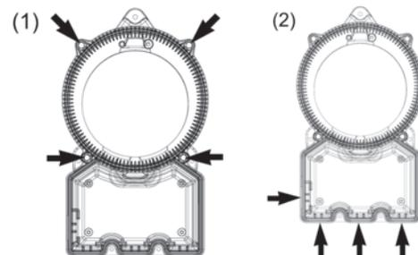
The MIX-4010-DUCT has one cable opening and provision for 3 more. See figure 10-2.
