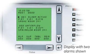
QS4 is as simple to operate as it is to set up. Its large 14-line backlit LCD display provides easy-to-understand details concerning up to 1,000 system events, while bright system status LEDs and large, tactile control buttons present the user with a clean, crystal clear interface. Four password levels limit control and information retrieval to authorized personnel. A priority access keyswitch gives Level 2 access, without a password, to management and emergency personnel.
