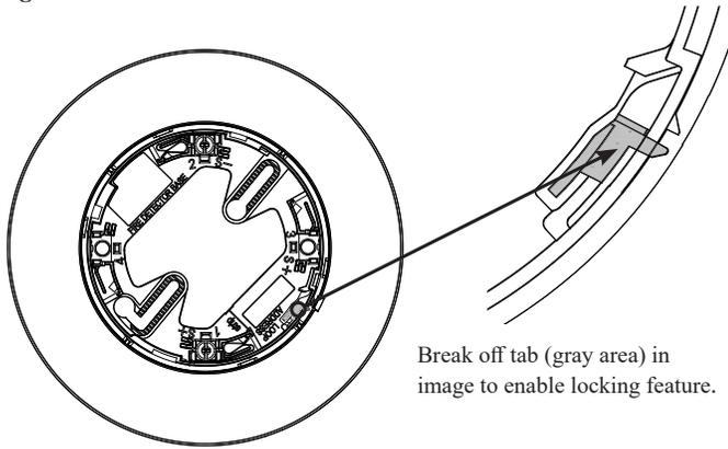
2. To remove the detector from the base when the locking feature has been enabled, insert a small screwdriver into the slot on the base to push the plastic tab while simultaneously turning the detector head counter-clockwise.
