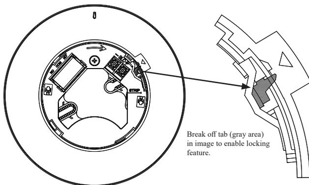
Removing of Detector Head from Base
