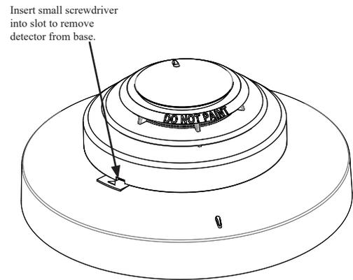
3. To remove the base cover from the lower enclosure once the locking feature has been activated, insert a small screwdriver into the slot on the base to push the plastic tab while simultaneously turning the detector head counter-clockwise.
